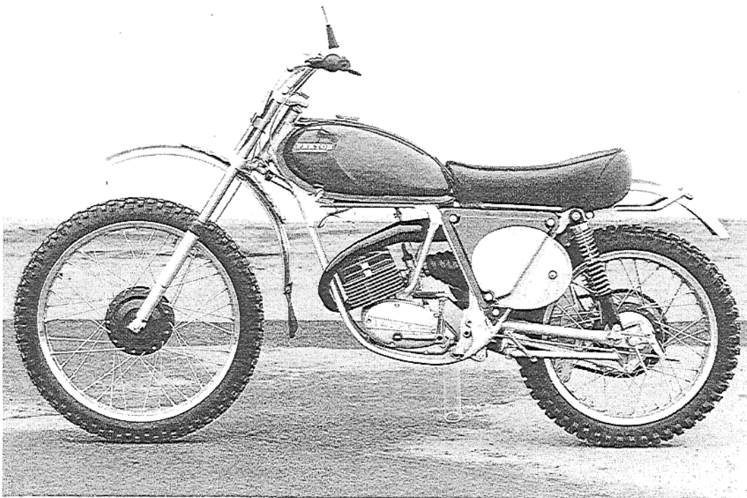
KTM prototype of a "Penton Junior Crosser" in a familiar CMF frame. Items shown that appear on the 1972 bikes are: The frame, air box cover, air boot, gas tank, seat, fenders, chain guard, exhaust pipe, side stand, and wheel assemblies. Items shown that were never used: front forks, swing arm with steel tanker style chain adjusters, the oval shaped Sachs motor, and the motor brace (which showed up on the KTM motors).
